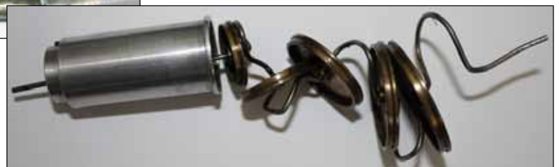
Bent drilling needle in telescope guidance of an IML-RESI M300
